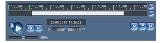
You will see a time bar below the video image for quick orientation. A green arrow above the bar indicates the position of the image currently being played back within the sequence. The time bar offers various options for navigation.
